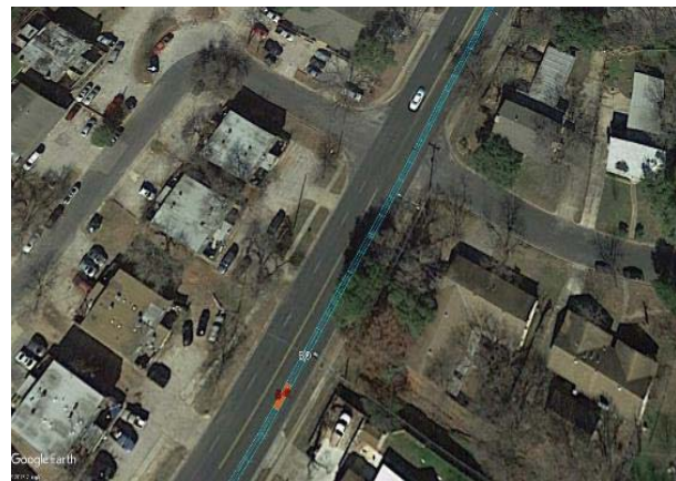
Figure 20: Geospatial GIS displays pipe-by-pipe location along with inspection results
