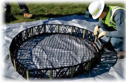
Figure 14: Capture Net for de-pressurized extraction
