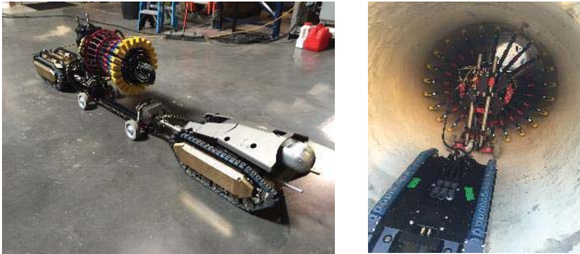
Figure 16 and 17: Robotic unit equipped with 24-detector EM array.
